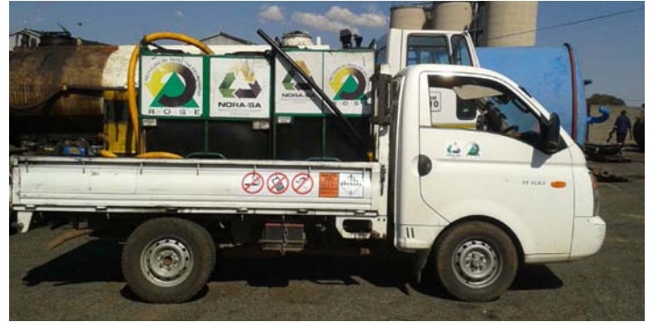
Example of a vehicle that exceeds the exempt quantity with the correct signage.
